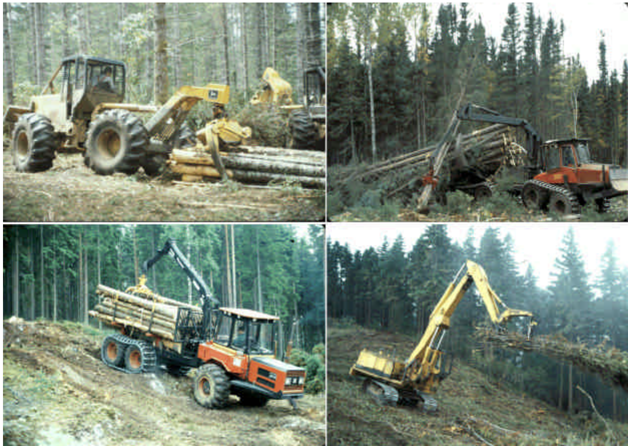
Figure 10.2. Ground-based equipment travels to the stump and brings logs/trees back to the landing. A wheeled grapple skidder (top left) can quickly grab bunches created by a feller-buncher, though a cable winch with chokers can replace the grapple in manually felled timber. A clam-bunk skidder (top right) can assemble and skid a much larger turn. A forwarder (bottom left) can collect a large turn from logs that have been felled and processed by a harvester. A shovel or log loader (bottom right) swings trees/logs towards the landing
