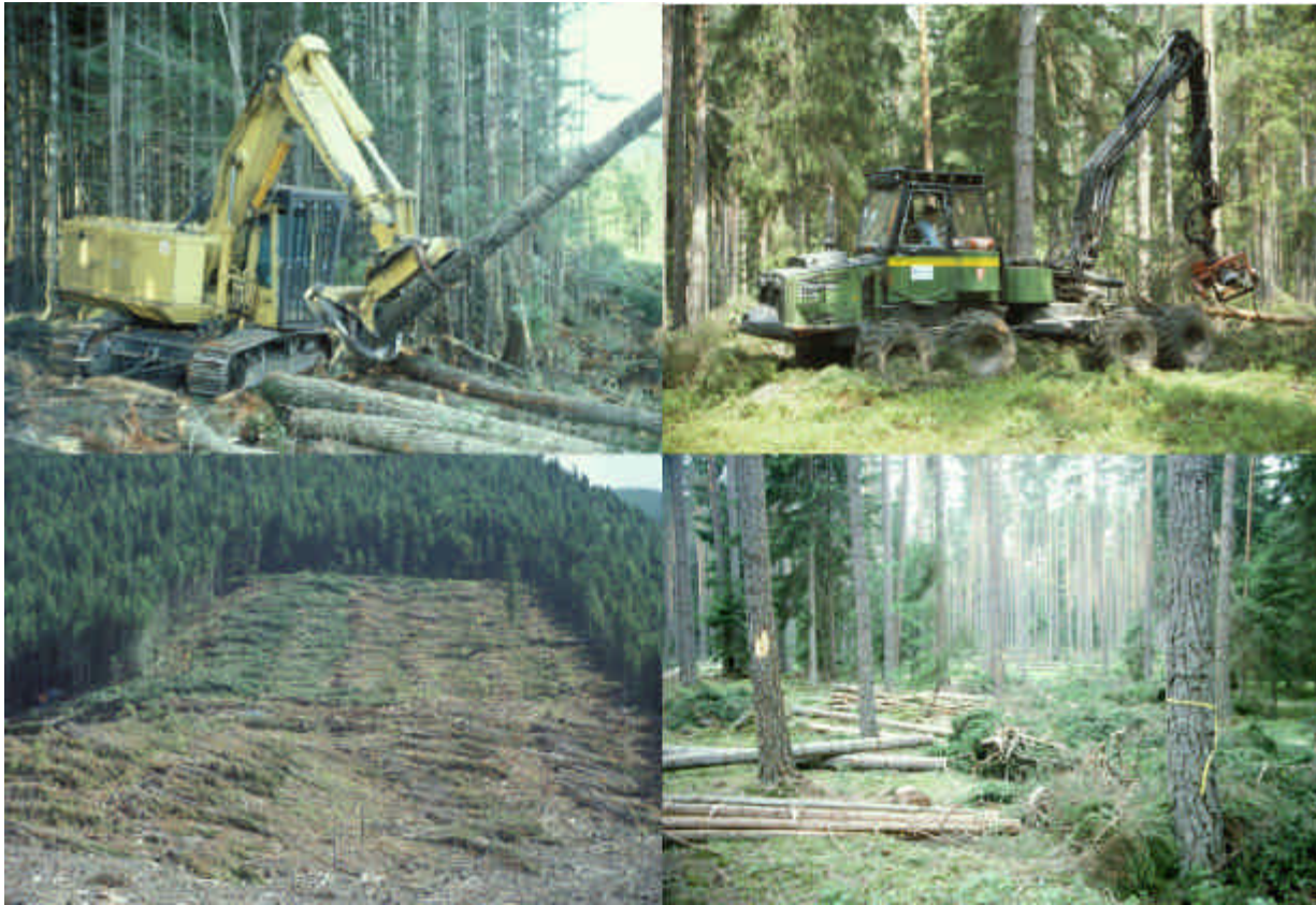
Figure 10.1 A feller-buncher (top left) fells trees into bunches (bottom left). A harvester (top right) fells and then delimbs and bucks the trees in its path, creating a slash mat that protects the soil. Logs are dropped in bundles or bunches to both sides of the yarding corridor (bottom right).
